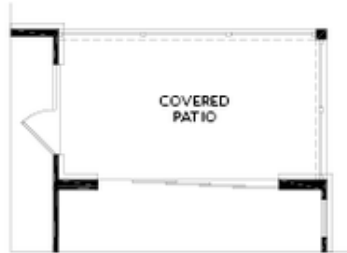
OPT Slider Door at Covered Deck
