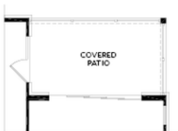
OPT Slider Door at Covered Deck
